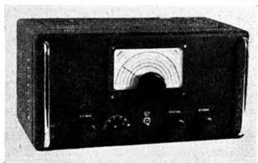
Front view of the receiver. Controls from left to right: A.F. Gain, Band Switch, Send-Receive Switch, Reaction and R.F. Gain.
